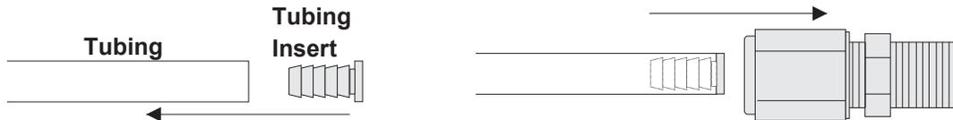
1. Insert tubing insert into I.D. of tubing (if required).
