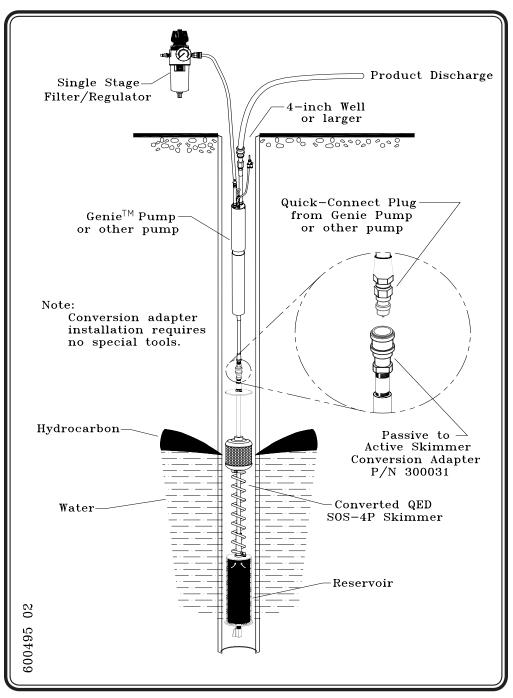
Figure 8 - Fully Automatic Product Recovery Upgrade with Genie Pump
