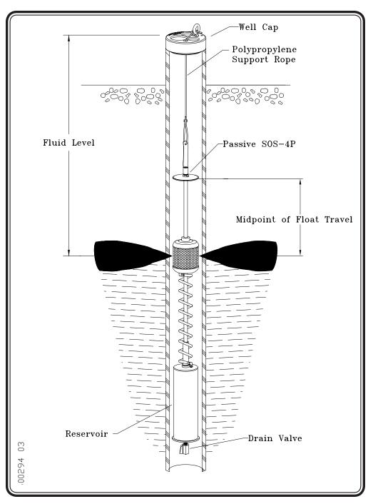
Figure 6 - Four-Inch Passive Selective Oil Skimmer (SOS-4P) Down Well
