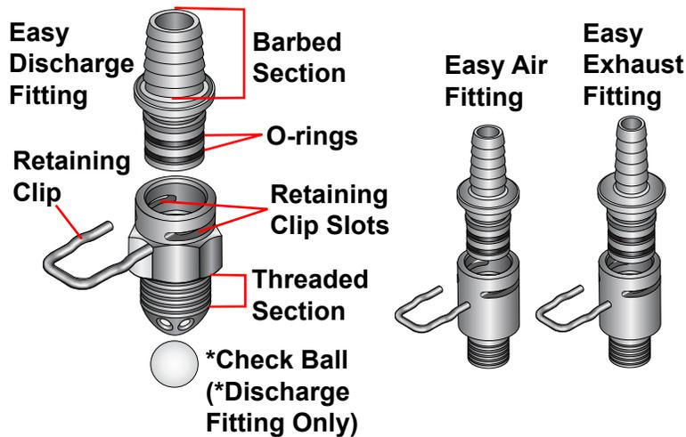
**IMPORTANT NOTE:** The smallest fitting is the air supply. This fitting needs to be threaded into the pump hole marked "I". The next larger fitting is the air exhaust fitting. This fitting needs to be threaded into the pump hole marked "E". If these two fittings are not installed into the correct holes the pump will not operate.
