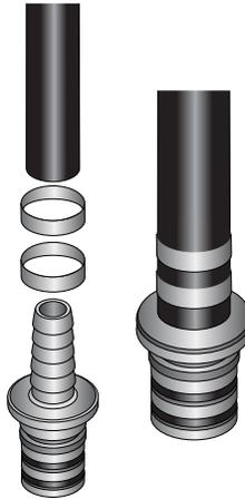
3. Wrap fitting threads with Teflon tape. Replace check ball in pump discharge (female) fitting before threading the Easy Fitting into it. Thread fittings into pump.
