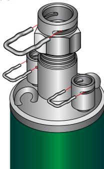
4. Insert male portion of fitting (with tubing attached) fully into its appropriate mating fitting on the pump.
