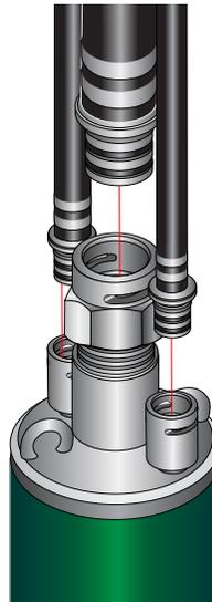
5. Push retaining clips into their mating retaining slots. Push clip into slot until it "clicks" into its locked position.
