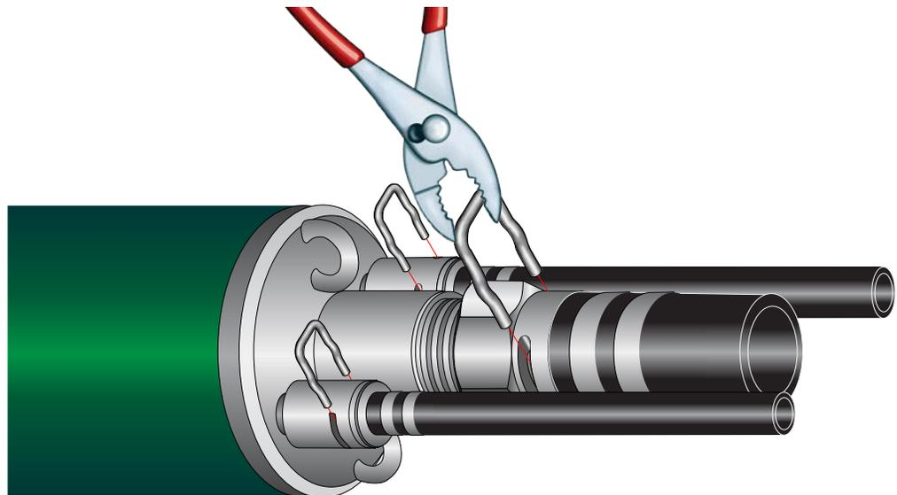
2. Tubing portion of the Easy Fitting should now be disengaged from the pump portion of the fitting and the tubing can now be pulled out and away from the pump. (See reverse side of this sheet, instructions # 4 & 5 for reassembling of fittings to pump).
