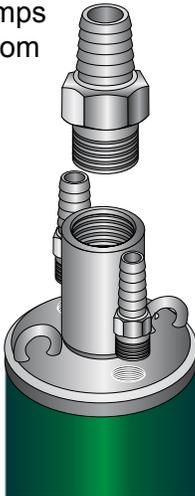
2. Slide tubing clamps onto tubing, then slide barbed portion of new fitting into tubing. Position clamps over barbed section of fitting. Clamp down clamps onto tubing using clamp tool. Use the same procedure for attaching the remaining fittings.
