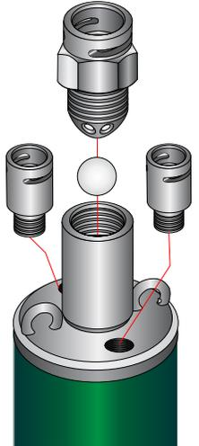
**NOTE:** Align retaining clip slots properly. When tightening fittings, tighten securely while keeping in mind the need to be able to easily access the fittings' retaining clips.
