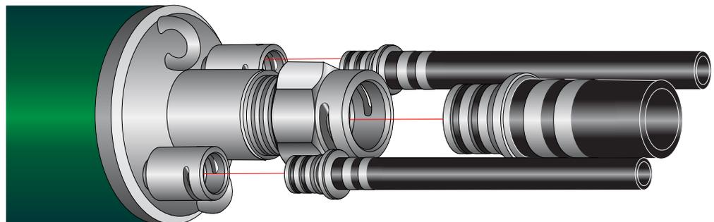
**NOTE:** Clean fittings, fitting clips and clip slots, inspect o-rings for damage (replace if necessary), before reassembling.
