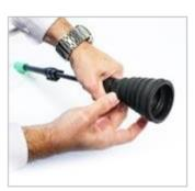
Unscrew and remove the rubber housing from the end of the sample probe.
