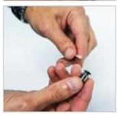
Remove the old tubing from the quickconnect fitting.
