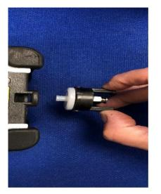
Change the filter and reassemble by turning it clockwise.
