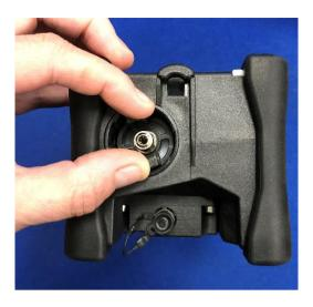
Unlock the filter by turning it counterclockwise and remove it.
