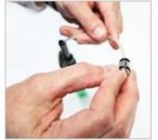
Connect the replacement tubing to the quick-connect fitting.
