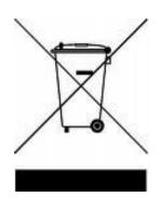
The wheelie bin symbol now displayed on equipment supplied by QED Environmental Systems Limited signifies that the apparatus must not be disposed of through the normal municipal waste stream but through a registered recycling scheme.
