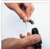
Hold the tube, unscrew the filter holder, and remove the quick-connect fitting from inside the filter holder.
