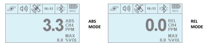
Note: The choice of absolute or relative mode is stored as non-volatile configuration. Each time the instrument is turned on, it will start using the same measurement mode it was using previously.
