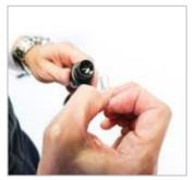
Remove the cellulose dust filter from the end of the filter holder.
