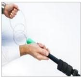
Remove the old tubing from the handle end of the sample probe
