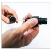
Unscrew and remove the nut at the top of the filter holder and remove the filter holder from the end of the sample probe.
