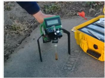
The FROG can also analyze soil samples onsite, detecting volatile organic compounds in soils down to part-per-billion level concentrations.
