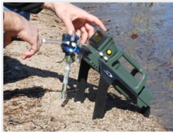
The FROG can detect volatile organic compounds in water as well. Water samples can be run onsite to reduce shipping and laboratory costs.
