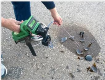
The FROG portable gas chromatograph can detect volatile organic compounds (VOCs) in air, delivering lab-quality results in less than 10 minutes.
