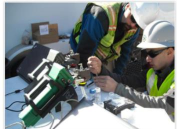
The FROG Portable GC can also be used to monitor your progress at remediation sites with quick, lab-quality results.
