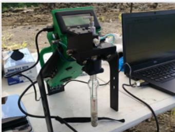
The FROG Portable GC is rugged enough to be used at the job site while attached to a computer or stand alone with results appearing on the display.
